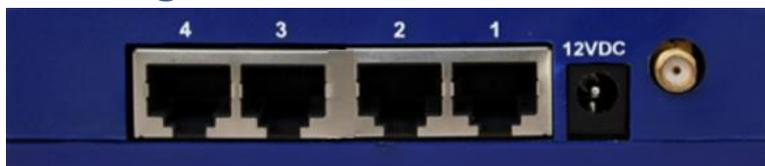
Port numbering starts from the power connector on the unit: the closest port to the power connector is Port 1 and closest to the Ethernet interface is Port 4.
