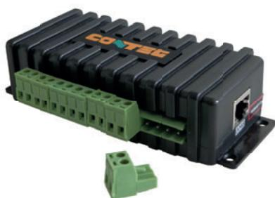
The expander allows creating 8 inputs/outputs on a single smart port of the main unit. Each port can be set as an input or output (output up to 20 mA). The expander's input contact is capable of supporting any type of door contact. The device is automatically recognized and powered from the main unit. The expander is connected using a standard LAN CAT 5/6 cable. Maximum cable extension length is 300 m.
