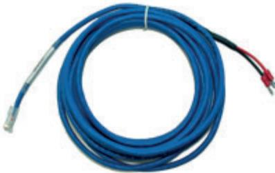
The dry contact sensor is used to connect external devices, such as security or fire systems, or any application that requires control by the unit. When used as an output, it can supply up to 20 mA. The input power supply range is 0 to 5 V. The contact is powered from the main unit. The extension is performed using a standard CAT5/6 network cable and an RJ45-RJ45 coupler RMS-I-CON. The maximum length of the extension cable is 300 m.
