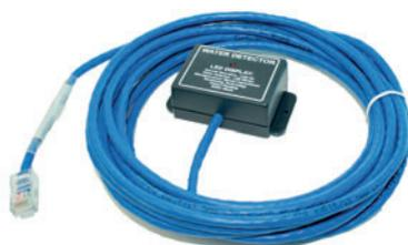
The spot water detector is able to detect water at the installation site. It has the possibility of LED indication on the device itself. Extension is done using a standard LAN CAT 5/6 cable. Maximum cable extension length is max. 60 m.
