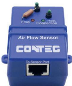
The sensor detects the presence or absence of flowing air inside the racks. The sensor works on the principle of differential measurement, which compares the resistance of the external and internal thermistor. This device can be connected to an alarm response and can be extended up to 30 m using a LAN CAT 5/6 cable.
