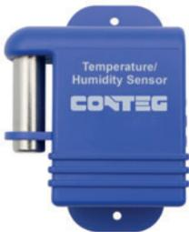
The encased temperature and humidity sensor is designed for placement inside racks and measures temperature in the range -55 °C to +75 °C and humidity in the range 0 to 100 %. The sensor can be extended for reach of up to 300 m using a LAN CAT 5/6 cable.
