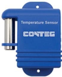
The temperature sensor is designed for placement inside racks and measures temperature in the range -55 °C to +75 °C. Up to 8 sensors can be chain linked to a single smart port. The sensor is powered from the main unit. Extension is done using a standard LAN CAT 5/6 cable. Maximum cable extension length is 150 m for 8 sensors.
