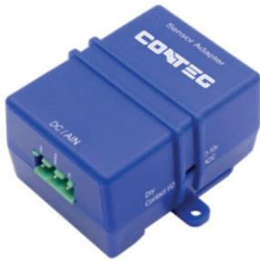
The Sensor Adapter makes it easy to connect 3rd party analog sensor with output 0-10 V DC. A switch on the side of the sensor adapter allows you to switch to a dry contact I/O instead, which is capable of maintaining a 5V DC output to power the sensor at all times, while still monitoring the dry contact input. This device is plugged into Optimax main monitoring units.
