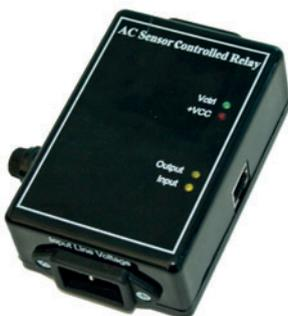
The AC-Sensor controlled relay allows you to control electrical devices over the internet. It monitors the power load and receives a control signal which is sent from the unit. The relay can provide automatic responses to sensor alerts. It has a built-in replaceable 10A fuse and is equipped with connectors C13 and C14. The relay can be controlled by any sensor. It is connected using a standard LAN CAT 5/6 cable with maximum connection length of 30 m.
