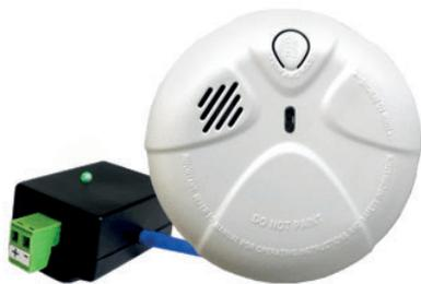
The detector emits an 85 dB two-state-alarm signal at a distance of 3 m from the unit and is also fitted with LED indication. It should be mounted on to the ceiling for maximum smoke detection ability. This device is powered from the main unit and can be connected to a back-up 9 V battery. It is connected using a standard LAN CAT 5/6 cable with maximum connection length of 90 m.
