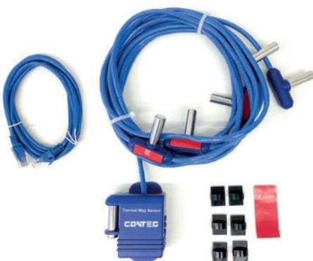
Thermal map sensors are ideal for complete environment monitoring in the racks. By using this device it is possible to determine hotspots and adjust the installation of IT hardware in the rack or regulate the output of the cooling unit. Pre-wired sensors on cable string monitor rack in 3 levels.
