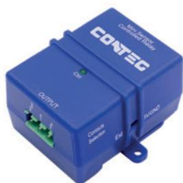
Mini Relay box with optional controlled power output can be plugged into RAMOS Plus or Optimax main monitoring units. This device can drive the larger relay with optional low current output. Equipment with a relay that needs to be switched based on sensor input, this adapter will switch contacts or output 200 mA – 5 V DC based on a sensor's status.
