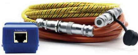
The rope water locating sensor is designed for specific location water detection. It can be connected to the main monitoring unit by intelligent sensor ports (RJ-45). This device is powered from the main unit. This sensor includes 3 m detection rope extendable via 3m extension detection cable, durable 6 m cable for connecting ropes to detector and detection module, main sensing module connected to intelligent LAN CAT 5/6 port via cable.
