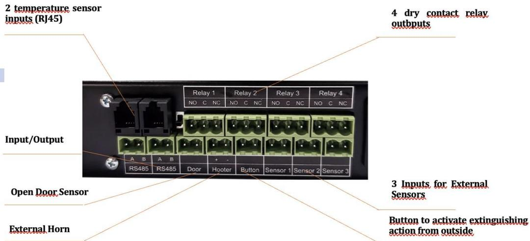
Figure number 4 - Description of the terminal board for connecting [Input/Output](#) devices
