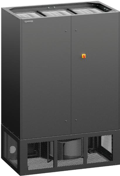
➤ **CRAC** indoor room cooling unit is based on the principle of compressor cooling and direct evaporation. The compressor is integrated into the indoor unit, which is connected to its external condenser unit.
