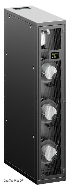
CoolTeg Plus DF in-row cooling units combine the advantages of CW and XC systems—free-cooling for low and medium outdoor temperatures and direct expansion cooling for use during high outdoor temperatures. The system thus reaches optimal minimum operating costs without the need to compromise.
